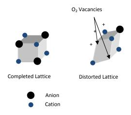
Figure 17. Illustration of completed and distorted lattices
