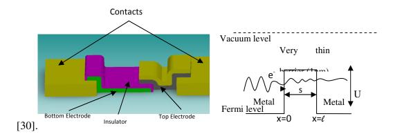
Figure 1. Side view of a typical MIM sandwich device
