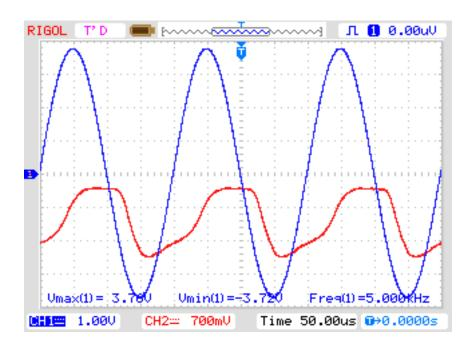
Figure 55. Rectification using the bilayer device at 5 kHz
