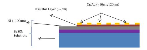
Figure 30. Side view schematic of the SK design
