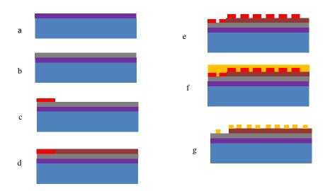
(a) SiO2 Substrate Conditioning (b) Blanket deposition of Ni (c) masking of the Ni layer for bottom electrode contact (d) deposition of NiO layer (e) masking of NiO layer for Cr/Au dots as top electrode (f) deposition of Cr/Au (g) removal of top electrode mask
