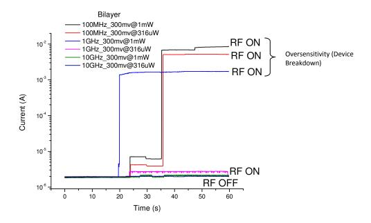
Figure 63. Detected current from Bi-layered devices
