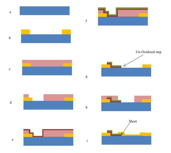
(a) SiO2 Substrate Conditioning (b) Pattern and deposition of Cr/Au Contact pads (c) spinning of photoresist (d) patterning of photoresist for bottom Ni electrode and NiO layer (e) deposition of Ni layer (f) deposition of NiO layer (g) liftoff (h) Spinning of photoresist and patterning for top electrode (i) deposition of top electrode.
