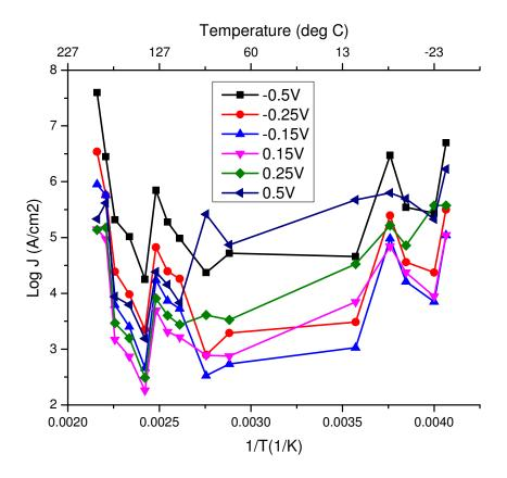
Figure 52. Plot of  $\log (J/V)$  as a function of temperature at different bias voltage of the Bilayer device.
