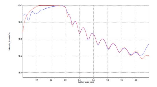
Figure 19. Fitted XRR spectrum of film deposited at  $20\%\,$  O2 partial pressure for 30 mins
