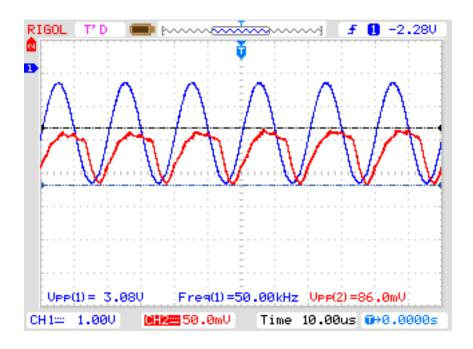
Figure 56. Rectification using the bilayer device at 50 kHz
