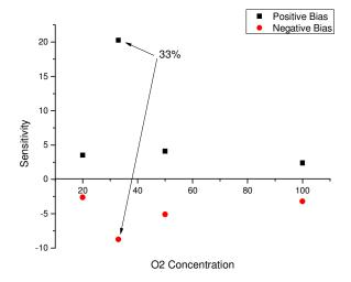
Figure 45. Sensitivities of the device plotted with respect to oxygen partial pressure
