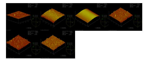
Figure 25. Starting from top left going clockwise, AFM images of NiO films deposited at 0%, 20%, 33%, 40%, 80%, 100%
