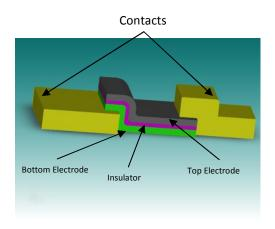
Figure 32. Sideview schematic of ST design
