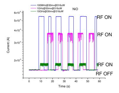
Figure 61. Detected current from NiO devices
