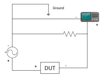
Figure 53. Schematic of the low frequency measurements setup
