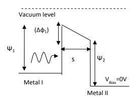
Figure 15. Energy band diagram of an MIM tunnel junction using two dissimilar metals
