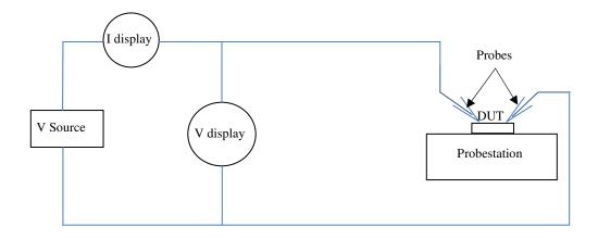
Figure 41. Schematic of the electrical measurement setup
