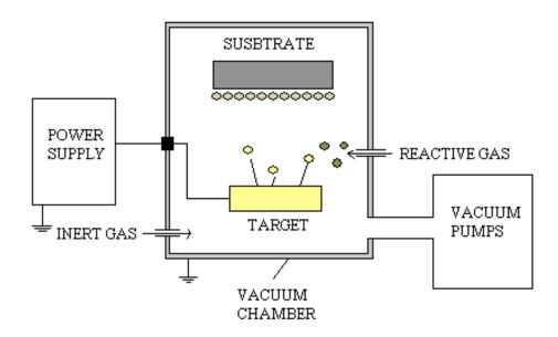
Figure 18. Schematic of a reactive sputtering process. Reprinted with permission [8]
