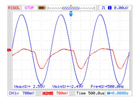
Figure 54. Rectification using the bilayer device at 500Hz
