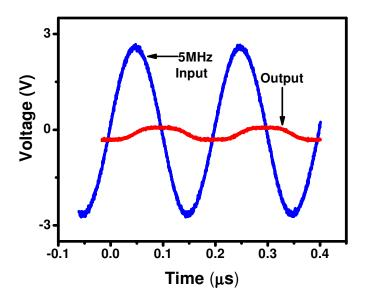
Figure 57. Rectification using the bilayer device at 5 MHz
