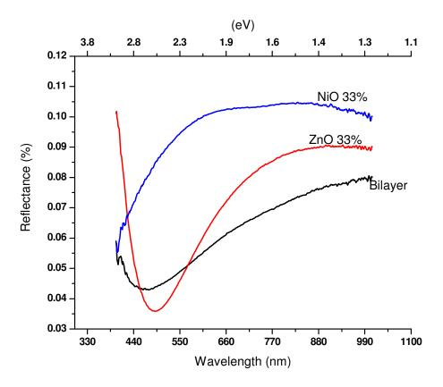
Figure 27. Reflectance mode UV-Vis spectra of NiO film, ZnO film and the bilayer film
