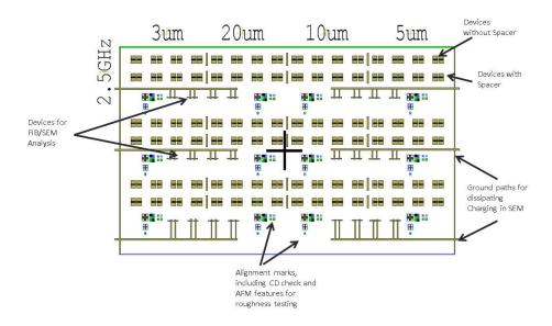
Figure 36. Overall layout of mask showing the functions of each feature
