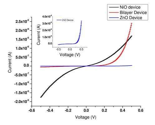
Figure 48. Comparison of I-V responses of devices fabricated with individual films as the insulator layer and the combination of the two.
