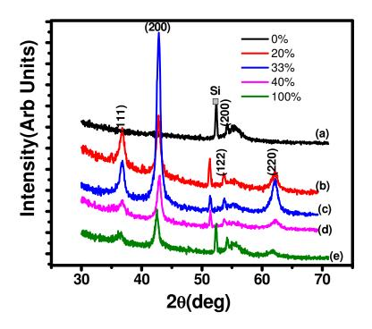
Figure 23. XRD spectra of films deposited with different Oxygen partial pressures. The 0% spectra is a Nickel only film.
