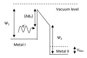
Figure 16. Energy band diagram of an MIM tunnel junction using two dissimilar metals at applied voltage Vbias
