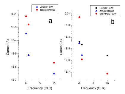
Figure 65. (a) Current vs frequency analysis of NiO, ZnO and bilayer devices with 1mW input power. (b) current vs frequency analysis of NiO, ZnO and bilayer devices with  $316\mu W$  input power
