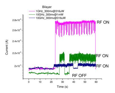
Figure 64. Closeup of the Bilayer devices at 1GHz and 10GHz with 1mW and  $316\mu W$  of input power
