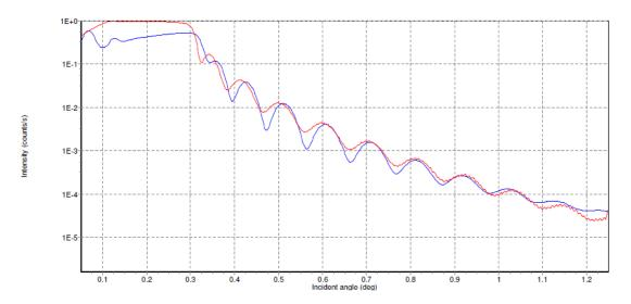
Figure 20. Fitted XRR spectrum of film deposited at  $33\%\,$  O2 partial pressure for 30 mins
