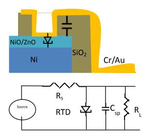
Figure 38. (top) Cross section schematic of parasitic capacitance due to spacer layer. (bottom) Equivalent circuit model of the same.  $R_s$  is the series resistance and  $C_{sp}$  is the parasitic capacitance due to the  $SiO_2$  spacer.
