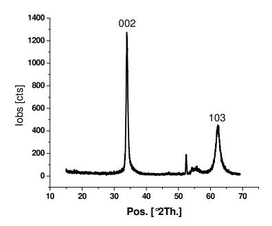
Figure 26. XRD spectrum of ZnO film showing strong c-axis orientation
