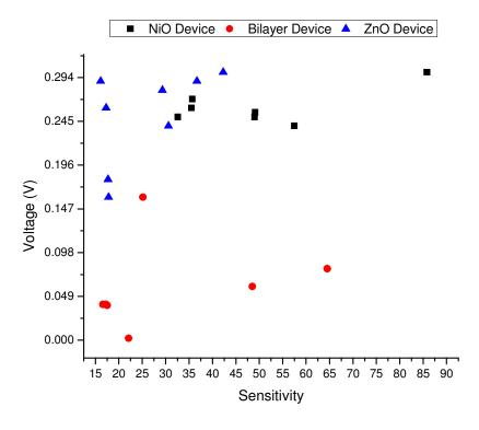
Figure 58. Comparison of sensitivity Vs turn on voltage of the NiO, ZnO and Bilayer based devices
