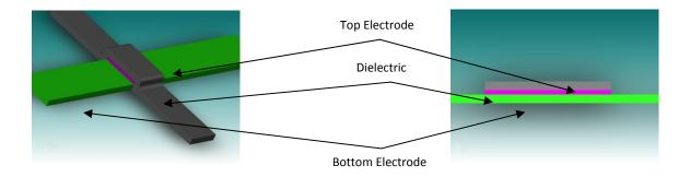
Figure 12. Crosshair type design of the tunnel junction
