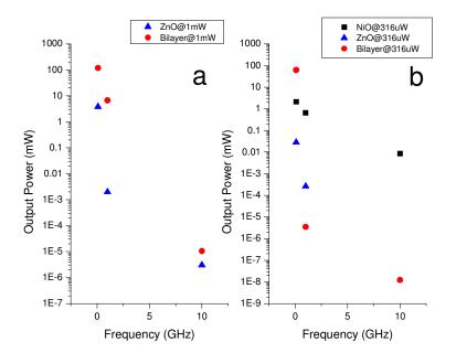
Figure 66. (a) Output power vs frequency analysis of NiO, ZnO and bilayer devices with 1mW input power. (b) output power vs frequency analysis of NiO, ZnO and bilayer devices with  $316\mu W$  input power
