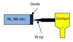
Figure 11. llustration of whisker diode
