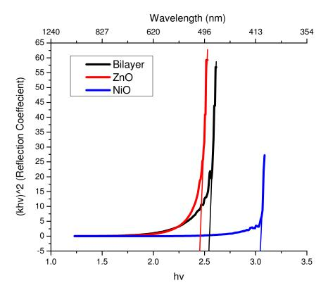
Figure 28. Band gap determination of NiO film, ZnO film and their combination
