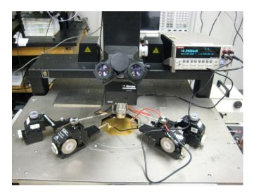
Figure 40. Cascade Probestation with Keithley 2400 Sourcemeter used to conduct DC measurements of the devices
