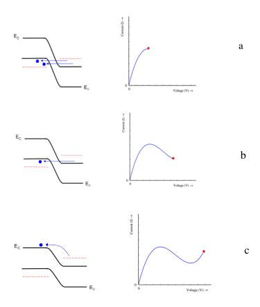
Figure 3. Working theory of semiconducting tunnel diodes [46-48]
