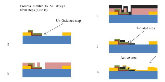
(g) liftoff after deposition of Ni layer and NiO layer (h) Spinning of photoresist and patterning for  $SiO_2$  spacer (i) deposition of spacer layer (j) liftoff (k) pattern, deposition and liftoff of top electrode revealing active area.
