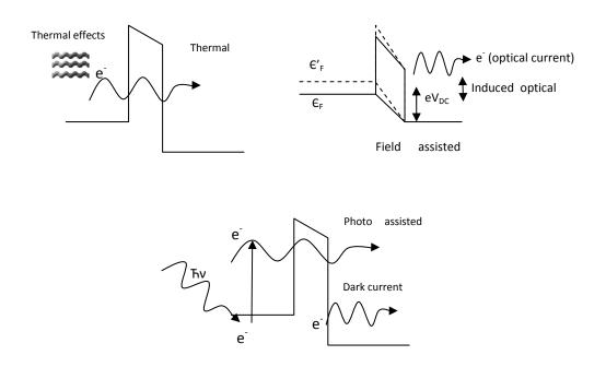
Figure 8. Illustration of different types of tunneling
